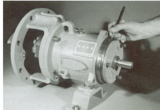
Example: For an impeller setting of 0.020 in (0.5 mm) off the casing, it is necessary to subtract 0.002 in (0.05 mm) for the movement caused by tightening the set screws; Therefore an adjustment of 0.018 in (0.46 mm) is needed. First, turn the bearing carrier clockwise until the impeller comes into light rubbing contact with the casing. Now rotate the bearing carrier counterclockwise 4-1/2 indicator patterns to get the 0.018 in (0.46 mm) clearance (0.004 x 4-1/2 = 0.018). FEOC
