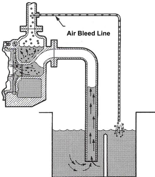
Normal operation commences as soon as the suction piping and the priming chamber are void of air (See FIGURE 6-4). Liquid from the impeller then passes through the discharge passage and into the priming chamber. At the same time, liquid from the impeller also passes through the bypass slot in the bottom of the casing and into the priming chamber. These two flows join and pass out of the priming chamber through the discharge nozzle located at the top of the chamber.
