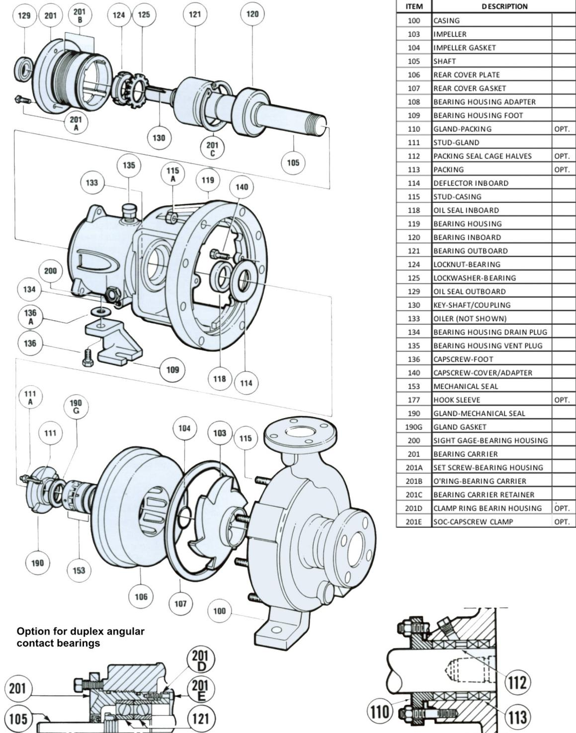
Option for duplex angular contact bearings
