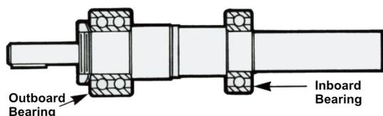
2. Place the snap ring (#201C for 1L and 2L type std.) or the bearing retainer (#201D for 3L type and 1L and 2L type with outboard duplex angular contact bearing) onto the outboard end of the shaft and slide down to the inboard bearing. Note the proper orientation of the bearing retainer or snap ring must be assured in this step. The flat side of the
